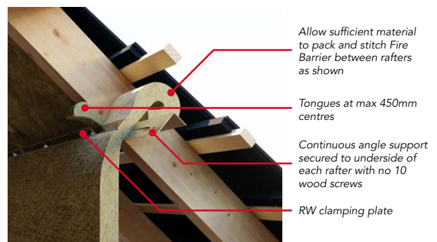
Figure 1 Fire Barrier traverse to rafters
